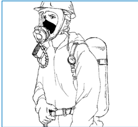
SCBAs provide air from a cylinder that is carried by the wearer.
