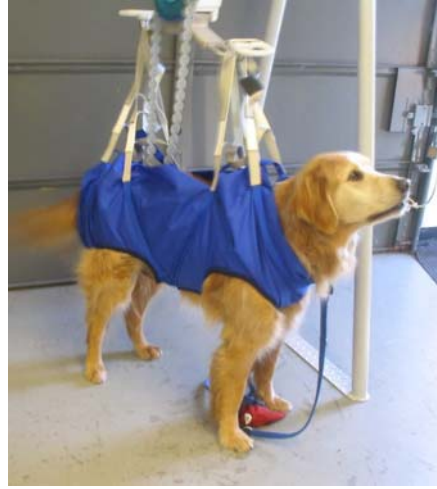
Pictures 7 a & b: Post-Clinical Trial Sling Design (Beta Prototype)
